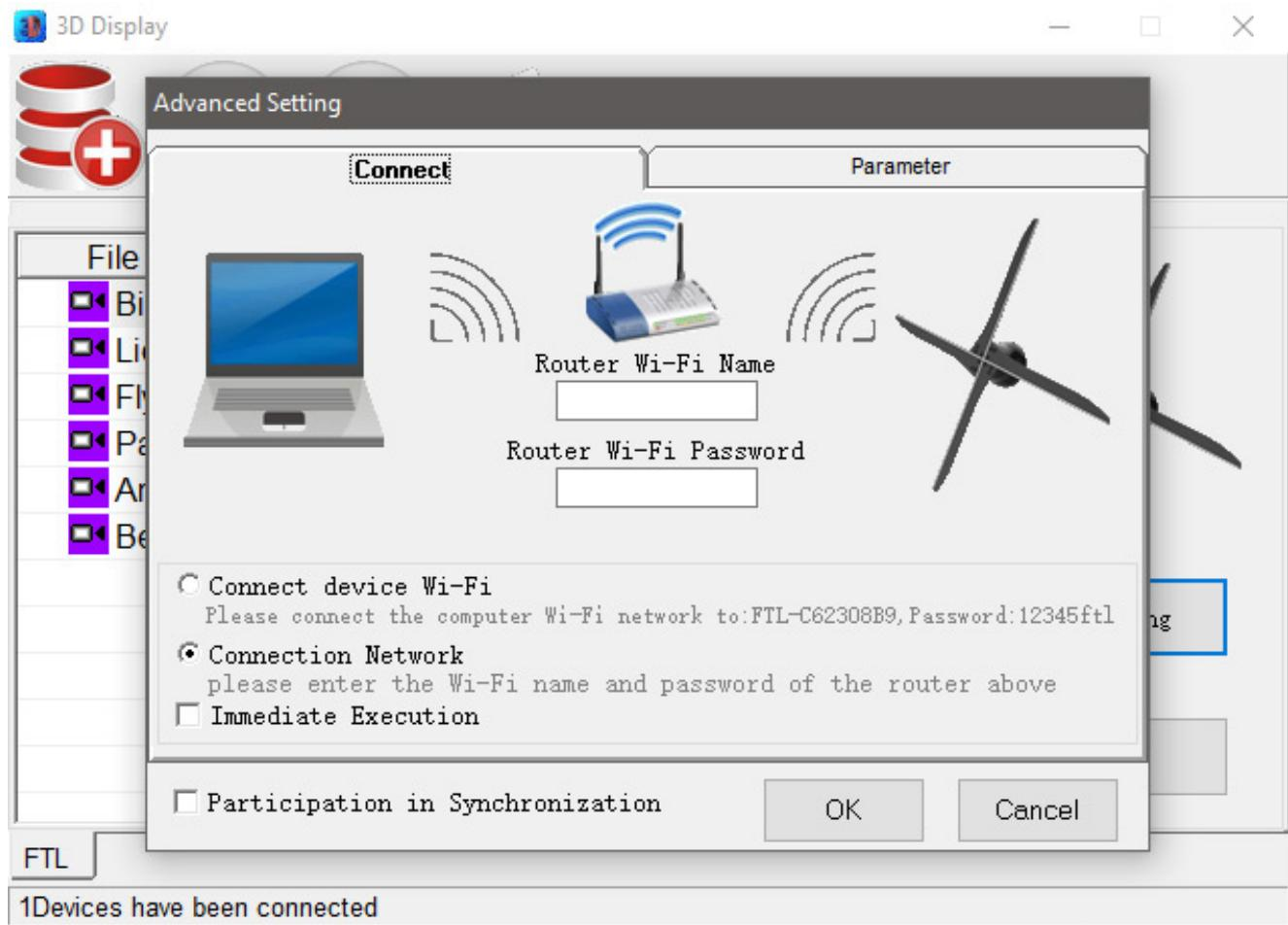
About two minutes later, the HotSpot FTL-XXXX (where XXXX is the number of your HoloRotor) will disappear and your device will automatically switch to the network of your router.
